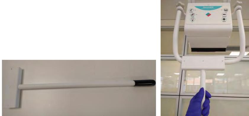
When it is not used, it can be placed on the back of the equipment.
