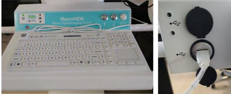
Place the 2D barcode reader on the support and connect it into the USB port found at the back of the unit, as shown below.
