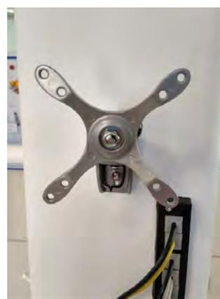
Use the Allen screws of 3 and 4 (CODE 64569 and CODE 62342) and the screws provided with the unit; rest the back of the PC on the support, aligned with the appropriate holes and tighten the screws as shown in the picture below.
