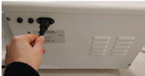
When you receive the unit, it is required to leave the battery charging for at least 12 hours before using the unit.
